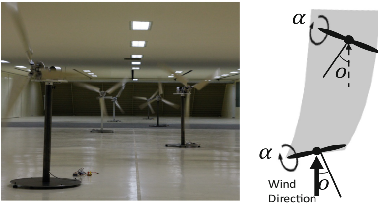
Fig. 7. Experimental wind tunnel set up with scaled wind turbines
