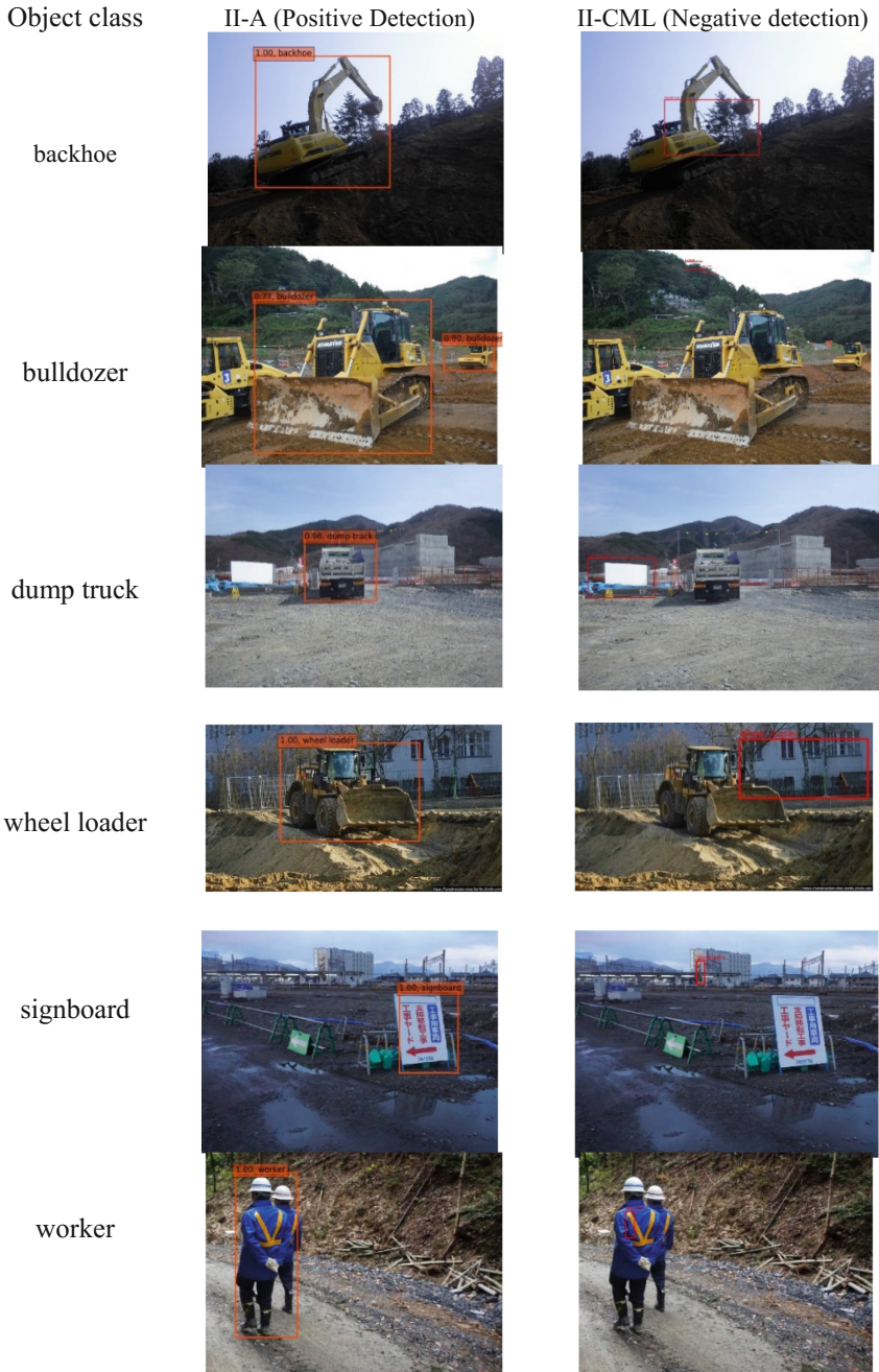
Fig. 8. Sample cases of positive detection by deep learning with transfer learning (II-A) and negative detection by conventional machine learning (II-CML).
