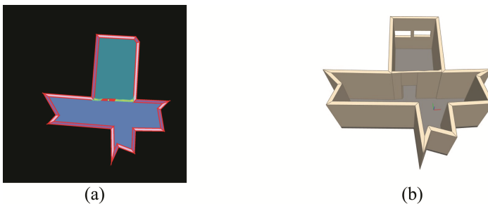
Fig. 8. Example dataset: showing (a) the resulting floor plan consisting of rooms, walls, doors and windows and (b) the automatically generated IFC model.
