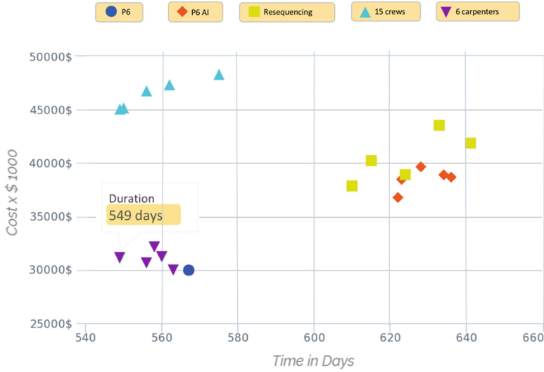
Fig. 4. Time-cost tradeoff chart produced automatically with the TCM. Each cluster of dots represents a different schedule scenario with the best five of the thousands of schedule options that are generated shown. For each dot, the corresponding 4D model, resource allocation, and other schedule information can be inspected.
