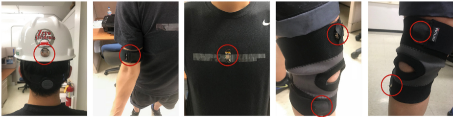
Fig. 2. Sensor placement (Head, Right arm, Chest, Right thigh, and Calf)
